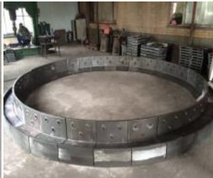
Kiln outlet nozzle
